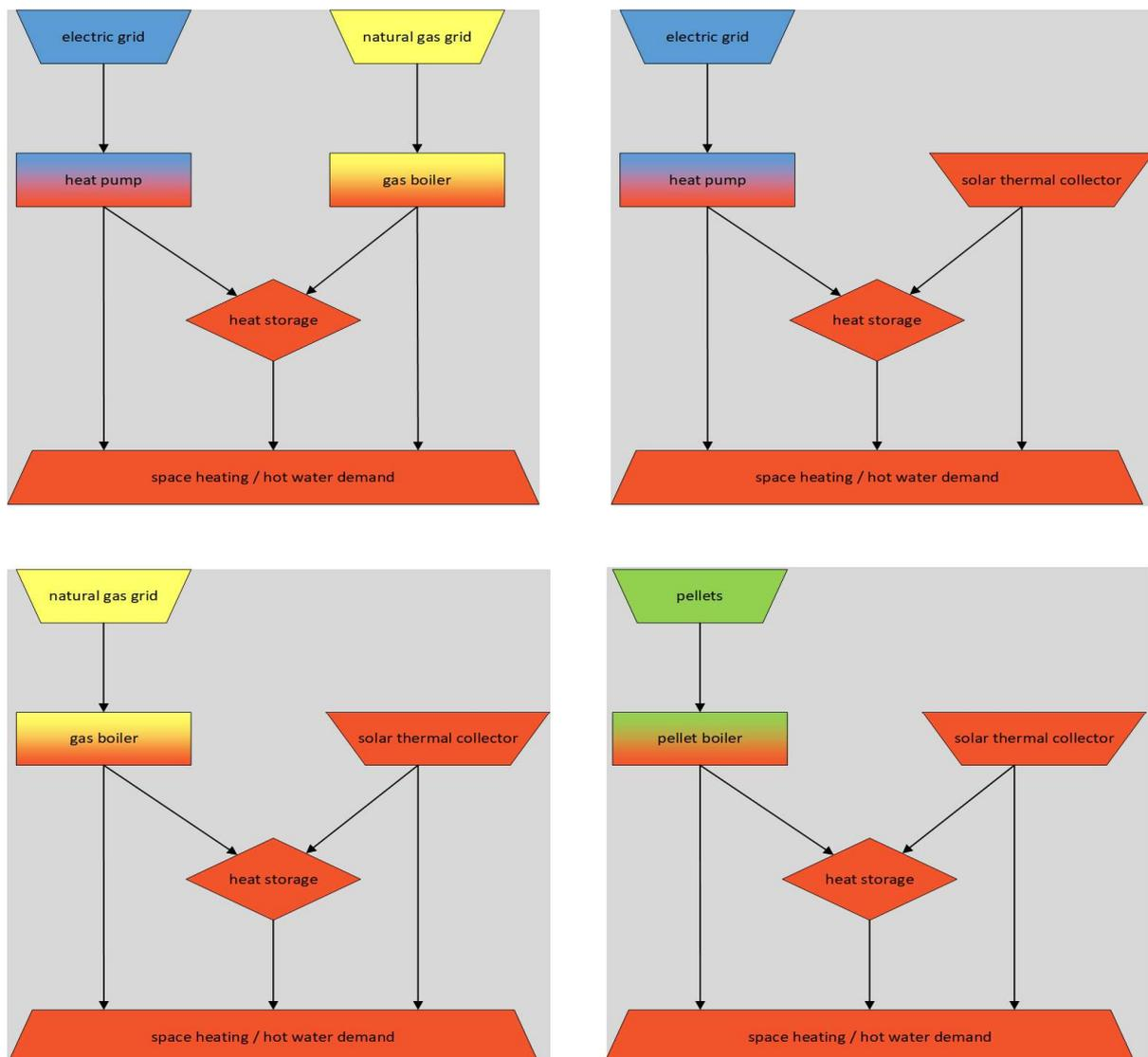
Figure 2: Energy flow graphs of the modelled energy systems. Upper left graph depicts S1, upper right S2, lower left S3 and lower right S4. The colour scheme indicates the respective energy sector: blue is the electricity sector, red the heat sector, yellow the gas sector and green the biomass sector.
